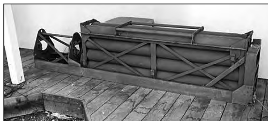
Figure 26.8 — An AB-577 temporary tower system in its transport case. (Photo by Alan Biocca, WB6ZQZ)
