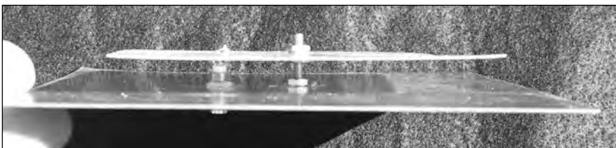
Figure 15.111 — An illustration showing how the patch is mounted above the ground plane using the center screw and, in this case, the SMA connector.
