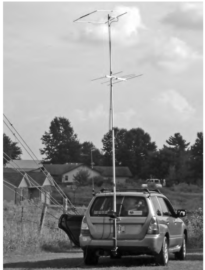
Figure 16.25 — A trailer-hitch bike rack can serve as a sturdy mount for an extendable mast such as this aluminum telescoping pole on NØAX’s car. The mast can be attached to the bike rack with U-bolts or brackets.
