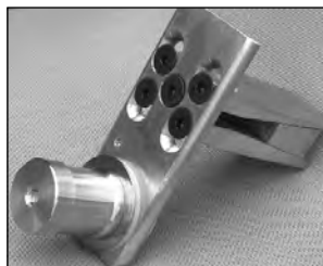
Figure 21.22 — A Scorpion 680 screwdriver antenna mounted on the truck of KG6PCI. (Photo courtesy of Alan Applegate, KØBG and Ron Douglass, N17J)
