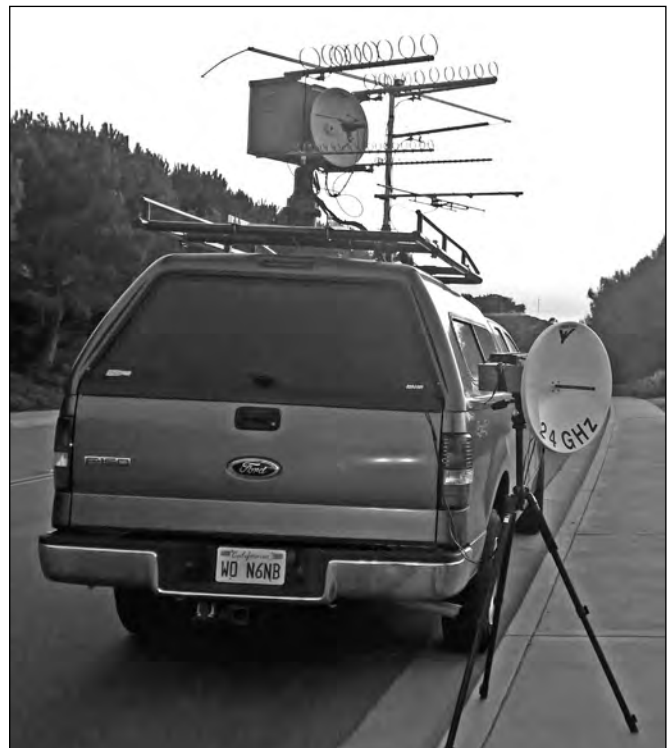
Figure 16.28 — N6NB's 11-band (6 meters through 24 GHz) mobile antenna farm is mounted on a frame attached to the vehicle's roof rack.
