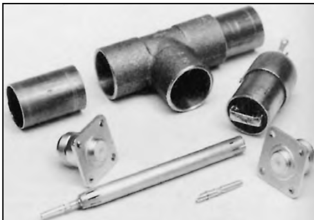
Figure 27.19 — Major components of the line sampler. The brass T and two end sections are at the upper left in this picture. A completed probe assembly is at the right. The N connectors have their center pins removed. The pins are shown with one inserted in the left end of the inner conductor and the other lying in the right foreground.
