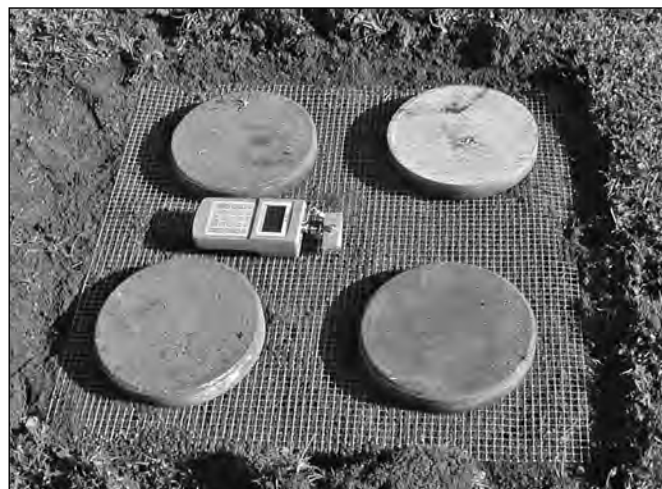
Figure 3.59 — Ground probe inserted through the mesh sheet.
