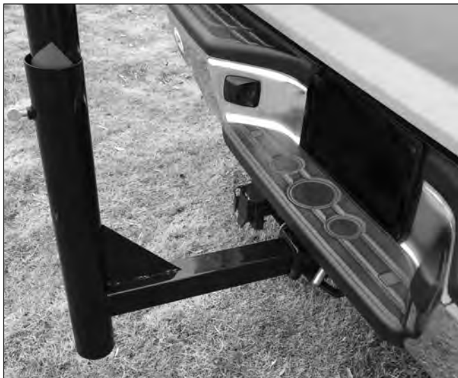
Figure 19.25 — K5ACL's welded mast mount attaches to a conventional trailer hitch receiver. [Courtesy Johnny Twist, K5ACL]
