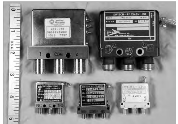
Figure 18.2 — Microwave coaxial relays with Type-N and SMA connectors.
