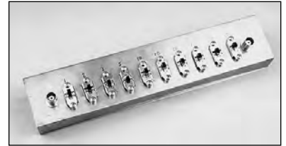
Figure 27.25 — The completed step attenuator in the enclosure of brass sheet. The BNC connectors may be mounted on the front panel at the end of the switches or on the end panels.
