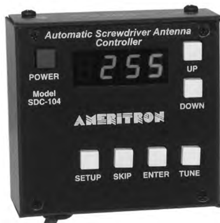
Figure 21.26 — A turns-counting controller keeps track of coil position by counting switch closures from a reed switch mounted on the antenna.
