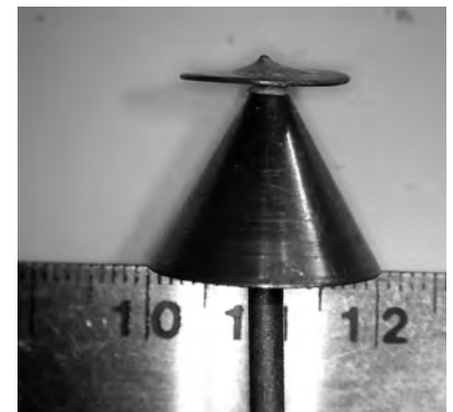
Figure 15.118 — An omnidirectional discone antenna for frequencies above 3 GHz made by Don Twombly, W1FKF.
