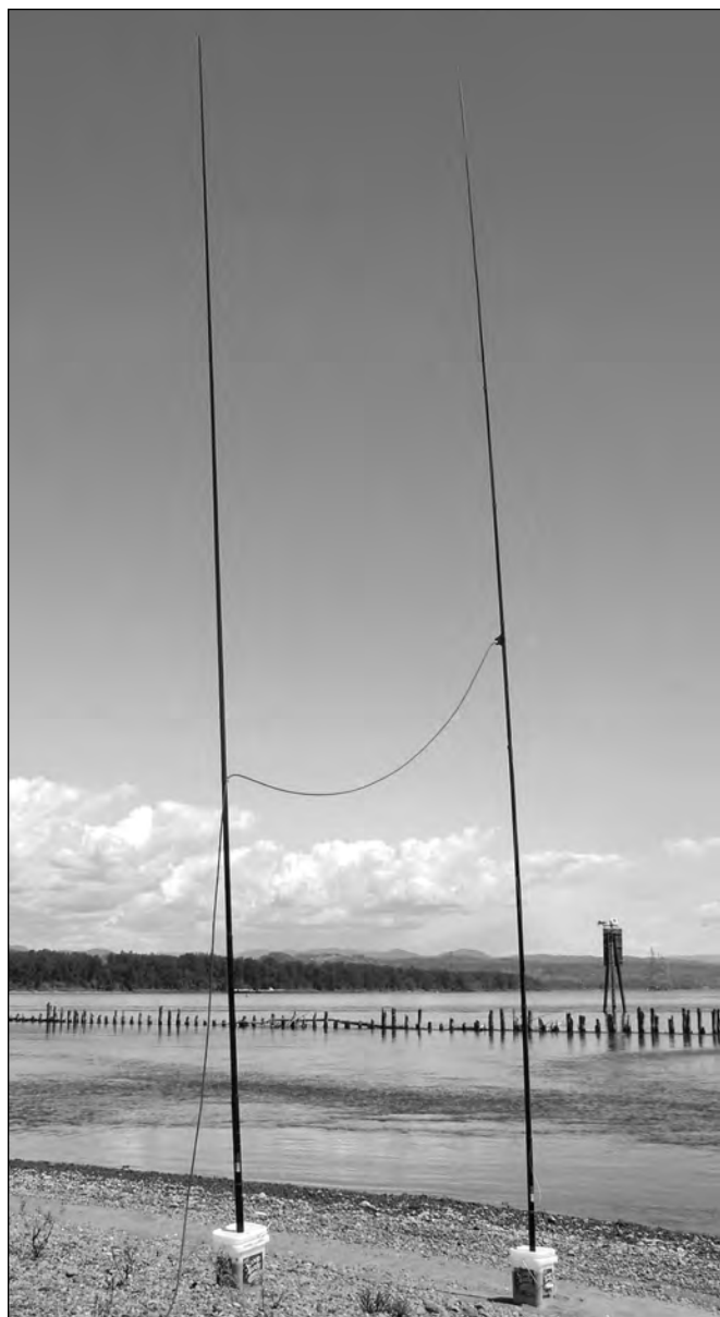
Figure 19.23 — A five-gallon plastic bucket filled with sand and rocks weighs from 40 to 60 pounds and makes a solid base for a fiberglass mast.
