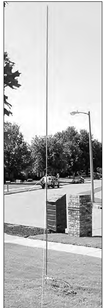
Figure 19.12 — The complete antenna set up in AD5X's front yard. Total height is about 16 feet.
