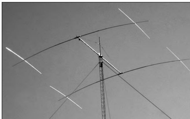
Figure 11.27 — A Cushcraft XM240 2-element 40 meter Yagi is modified by W6NL to become a Moxon Rectangle. The antenna is mechanically strengthened during the modification, as well. (Photo by Dave Leeson, W6NL)
