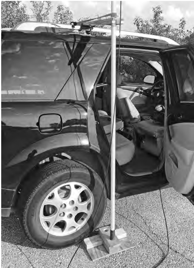
Figure 16.24 — A simple “drive-on” mount for a painter’s pole or other inexpensive mast. A strut attached to K5ND’s vehicle roof rack secures the mast at about head height.
