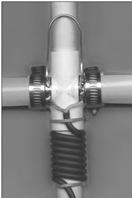
Figure 22.48 — Photo of driven-element mounted to PVC tee using hose clamps. The hairpin match wires are shown here soldered to the tape-measure elements, along with the RG-58 feed line.
