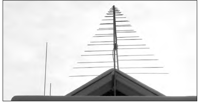
Figure 15.60 — The Tennadyne T-28 covers 50-1300 MHz with boom length of 12 feet.
