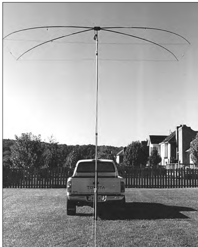
Figure 19.20 — The completed 15 meter beam mounted on a painter's pole mast.
