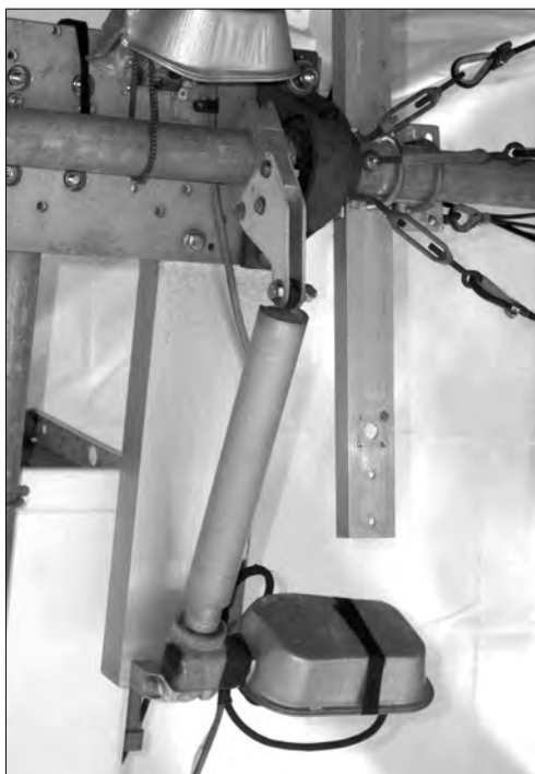
Figure 17.40 — KD1K’s homebrew elevation rotator drive using a surplus-store drive screw mechanism. Note also the large journal bearing supporting the elevation axis pipe shaft. [Dick Jansson, KD1K, photo]
