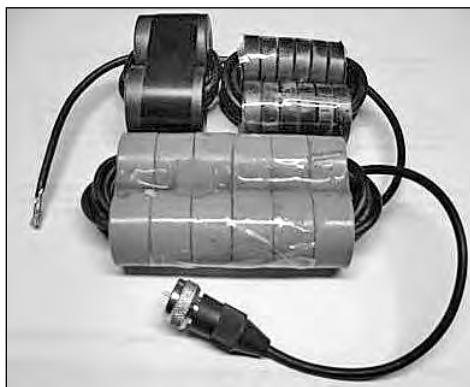
Figure 22.13 — The coaxial common-mode choke, used on each antenna termination.
