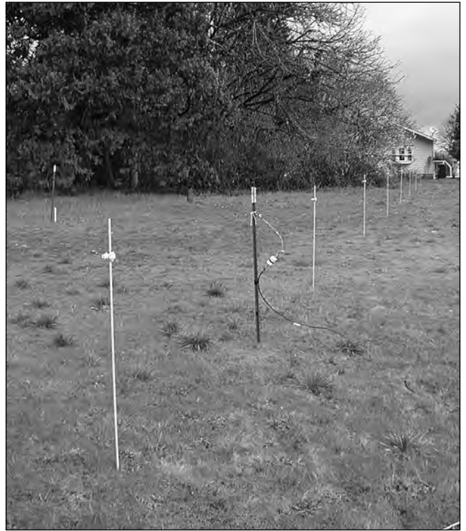
Figure 3.64 — Test antenna supported with fiberglass wands.
