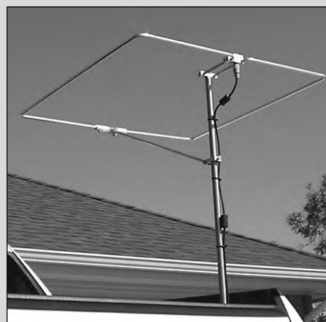
Figure 16.A — A squalo (square halo) is a popular horizontally polarized VHF/UHF mobile antenna.
