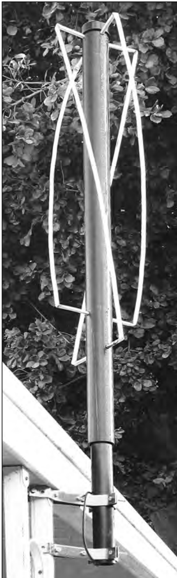
Figure 17.18 — W6NBC's Quadrifilar Helix base station antenna [John Portune, W6NBC, photo]
