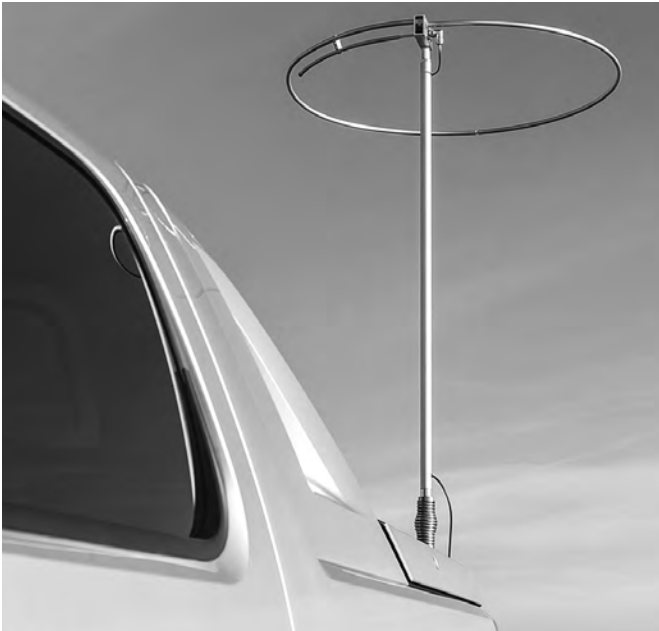
Figure 16.18 — A 6 meter halo antenna can be used as a mobile antenna if carefully constructed. The antenna shown here was designed and built by Jerry Clement, VE6AB.
