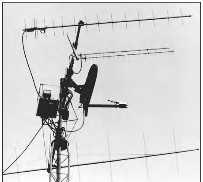
Figure 17.25 — Details of KD1K's tower cluster of satellite antennas including a home-brew elevation rotator. Top to bottom: M2 436-CP30, a CP U-band antenna; two M2 23CM22EZA antennas in a CP array for L band; “FABStar” dish antenna with helix feed for S band; M2 2M-CP22, a CP V-band antenna (only partially shown.) To left of dish antenna is a NEMA 4 weatherproof equipment box with an internal 40-W L-band amplifier, and also hosts externally mounted preamplifiers. (KD1K photo)
