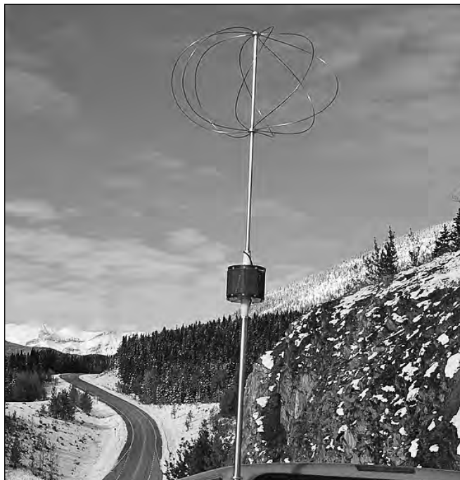
Figure 21.20 — A "bug catcher" style antenna showing the large, air-wound center-loading coil in the center of the antenna with a capacitance-hat at the top. This antenna was designed and constructed by VE6AB.
