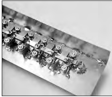
Figure 27.24 — The attenuator before final mechanical assembly. The ¼-inch strips are spaced 0.033 inch apart to form a 50-Ω connection from the BNC connector to the stripline. There are ½-inch square shields between 10-dB sections. The square shields have a notch in one corner to accommodate the end of the rectangular tubing.
