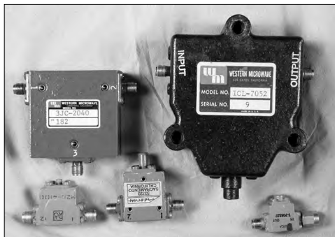
Figure 18.7 — Typical isolators and circulators. Largest is for 1296 MHz. Circulator marked “3JC-2040” indicates that it covers 2.0 to 4.0 GHz. Small isolators all work at 10 GHz.
