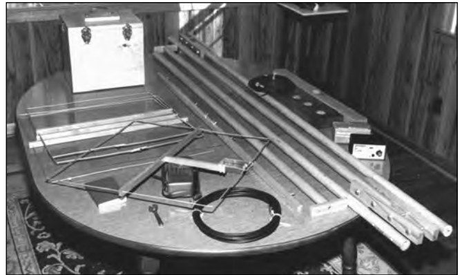
Figure 15.52 — The complete portable quad, broken down for travel. Visible in the foreground is the driven element. The pine box in the background is a carrying case for equipment and accessories. A hole in the lid accepts the mast, so the box doubles as a base for a short mast during portable operation. (W1MPO photo)
