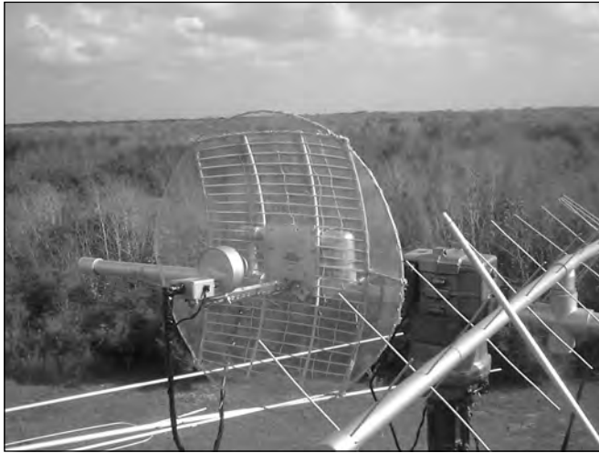
Figure 17.34 — K5GNA's "circularized" mesh modification of an MMDS dish antenna with a helix-CP feed and preamp. The dish modification reduces the spillover loss by making the antenna fully circular. [Gerald Brown, K5OE, photo]
