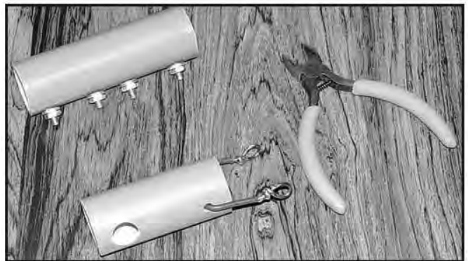
Figure 10.21 — Insulators can also be made from inexpensive PVC pipe. At the top is a feed point insulator for parallel-conductor feed lines. The feed line is attached to the inner terminals and the loop to the output terminals which are jumpered together (jumpers not shown). At the bottom is a corner insulator. The support line is tied through the larger holes and the loop conductors attached to the eyes of the jumper.
