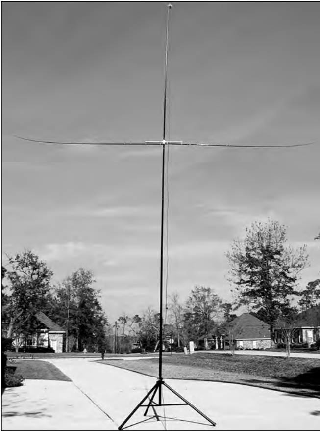
Figure 19.4 — The portable inverted-V antenna is built using a lightweight fiberglass support mast and two fishing poles. No additional supports are required and the antenna can be moved and rotated by hand.
