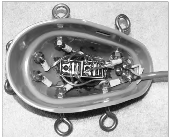
Figure 13.35 — Relay box assembled in a power entry PVC cover.
