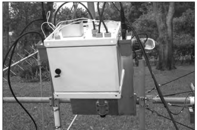
Figure 18.22 — A NEMA 4 box is used to shelter the L-band band electronics and power supply. The box flanges are convenient for mounting preamplifiers. The box is shown inverted since it is on a tilt-over tower.
