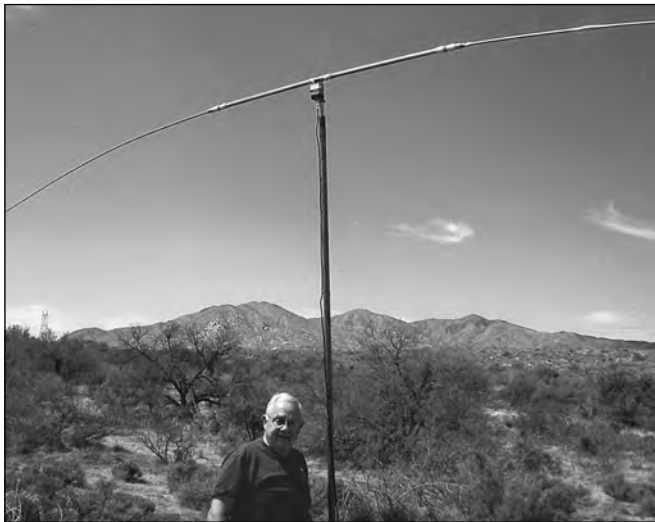
Figure 19.7 — This portable dipole uses a fixed center section and extendable telescoping whips to adjust the resonant frequency.
