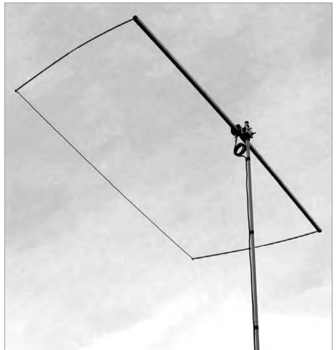
Figure 16.23 — The stressed Moxon SM-50 by PAR Electronics is a Moxon rectangle designed with the forward element under tension. The resulting lightweight construction is robust under rover conditions.
