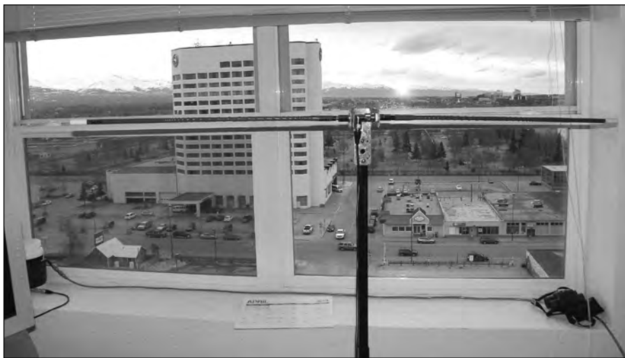
Figure 20.10 — This pair of CB mobile antennas were trimmed slightly to resonate on 10 meters then attached to a mounting bracket. This created an effective apartment-sized antenna.
