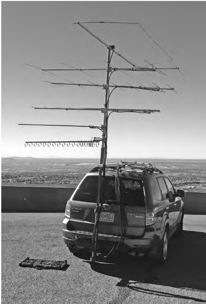
Figure 16.26 — Heavier trailer-hitch masts can support several antennas. This mast for KK6MC's rover is supported by a strut attached to the roof rack.
