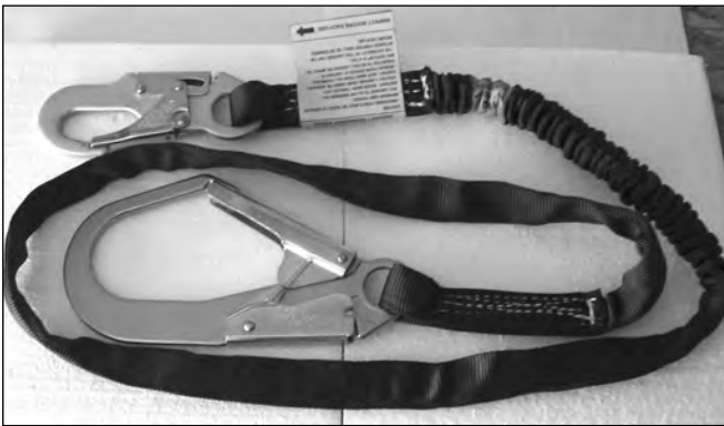
Figure 26.3 — A shock absorbing fall arrest lanyard. Portions of the nylon webbing are sewn together and pull apart under the weight of a climber falling on it, thus decelerating the fall.
