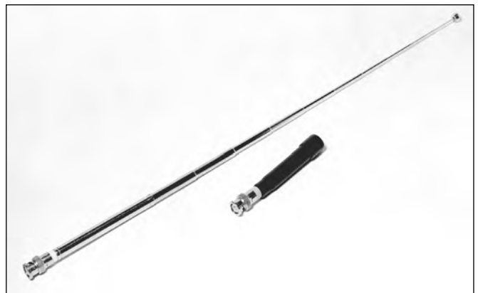
Figure 16.1 — A telescoping \frac{1}{4} -wavelength antenna and a flexible “rubber duck” antenna, both designed for use on 2 meters. The telescoping antenna is approximately 19 inches long when extended, while the flexible antenna is only 3\frac{1}{2} inches long. The flexible antenna is a helically wound radiator used because of its mechanical strength.
