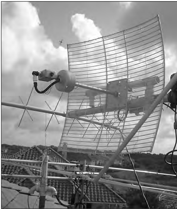
Figure 17.35 — Mesh modification of an MMDS dish antenna by K5OE, with a helix-CP feed and preamplifier by Down-East Microwave mounted directly to the helix feed point. [Gerald Brown, K5OE, photo]
