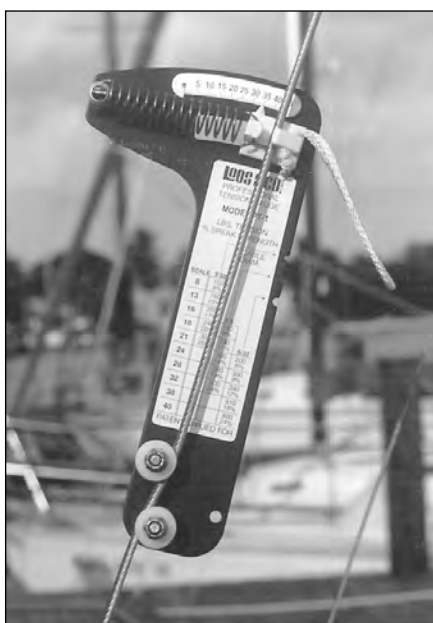
Figure 26.41 — Loos PT-2 guy wire tension gauge.
