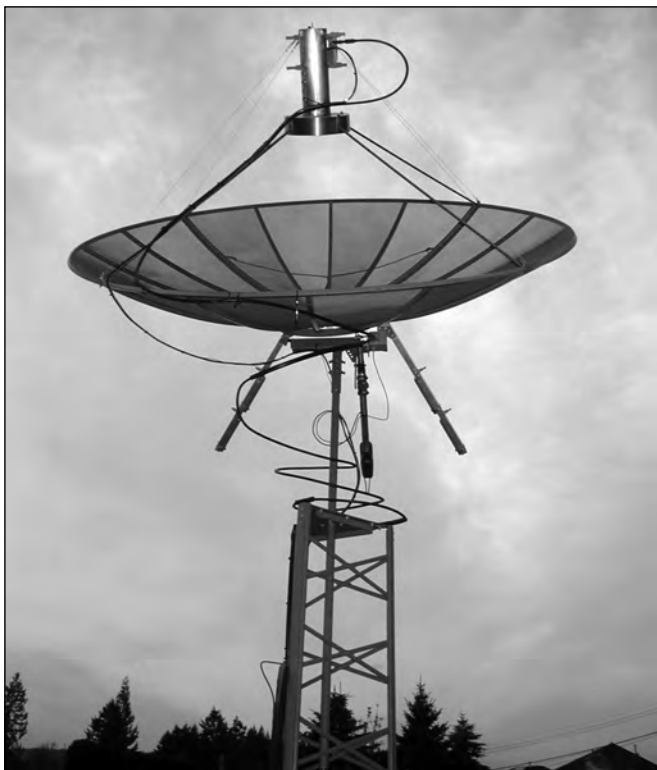
Figure 17.30 — This 3-meter TVRO dish with aluminum frame and mesh surface was outfitted for 1296 MHz EME as a joint effort by VA7MM and VE7CNF. The dual circular polarization feed is a VE4MA/W2IMU design.
