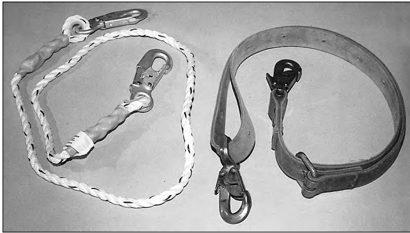
Figure 26.2 — A fixed-length rope positioning lanyard on the left and a versatile Klein adjustable lanyard on the right. They both use double-locking snap-hooks.
