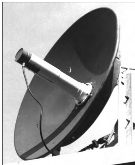
Figure 15.88 — Coffee-can 2304 MHz feed described in text and Figure 15.85 mounted on a 4-foot dish.
