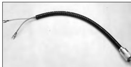
Figure 24.61 — W2DU bead balun consisting of 50 FB-73-2041 ferrite beads over a length of RG-303 coax. See text for details.
