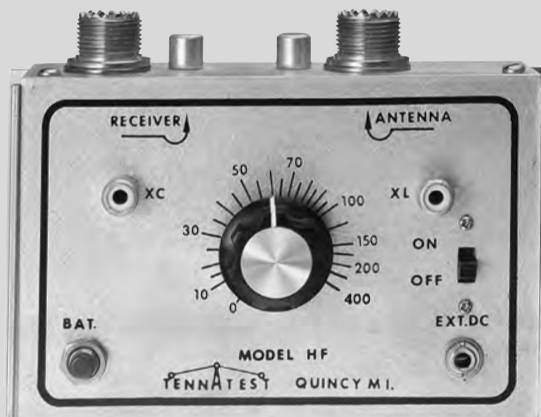
Figure 27.30 — A noise bridge is an alternative to the antenna analyzer, pairing a noise source with an external receiver as the detector. The bridge is adjusted for minimum noise in the receiver and values for R and X are read from calibrated dials. An article on using the noise bridge is downloadable with this book's supplemental information.
