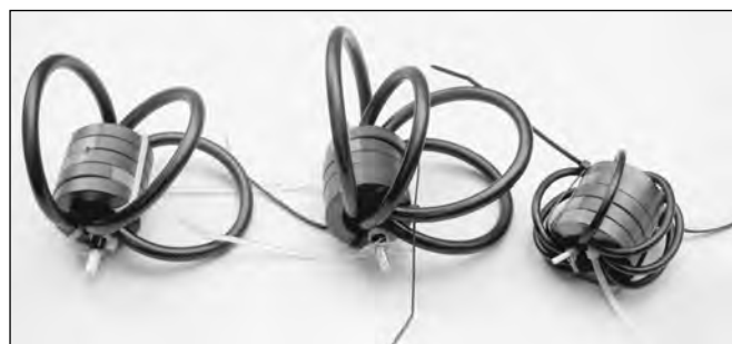
Figure 24.57 — Legacy design coax-wound ferrite transmitting chokes for use on the HF bands. Figure 24.59 shows examples of currently recommended choke construction.
