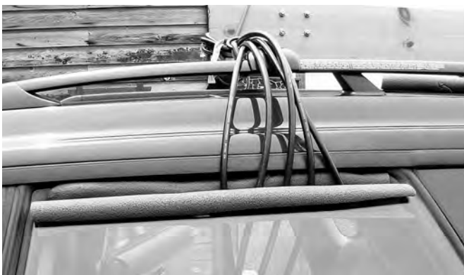
Figure 16.29 — An inexpensive "pool noodle" makes a coax-friendly window seal for getting feed lines into and out of KK6MC's vehicle. Slit the foam along one side, slide it over the window, and raise the window until the foam seats around the cables.
