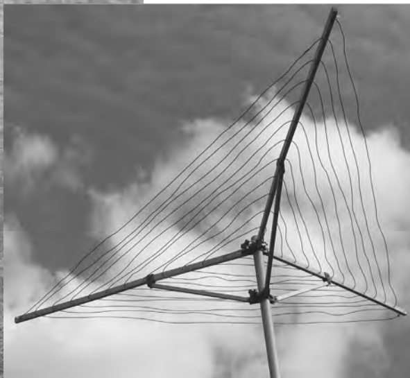
Figure 20.14 — Martin, G8JNJ, converted a scrap laundry drying rack into a stealthy HF vertical. At A is the complete antenna showing the top and bottom counterpoise and capacity hat, respectively. B shows the upper capacity hat. [Photos courtesy of the RSGB and Martin Ehrenfried, G8JNJ]
