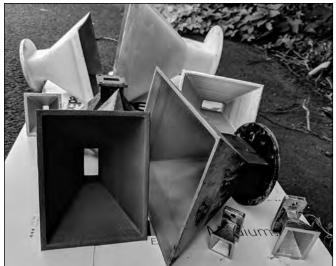
Figure 15.81 — 3D-printed horns before and after metalization.
