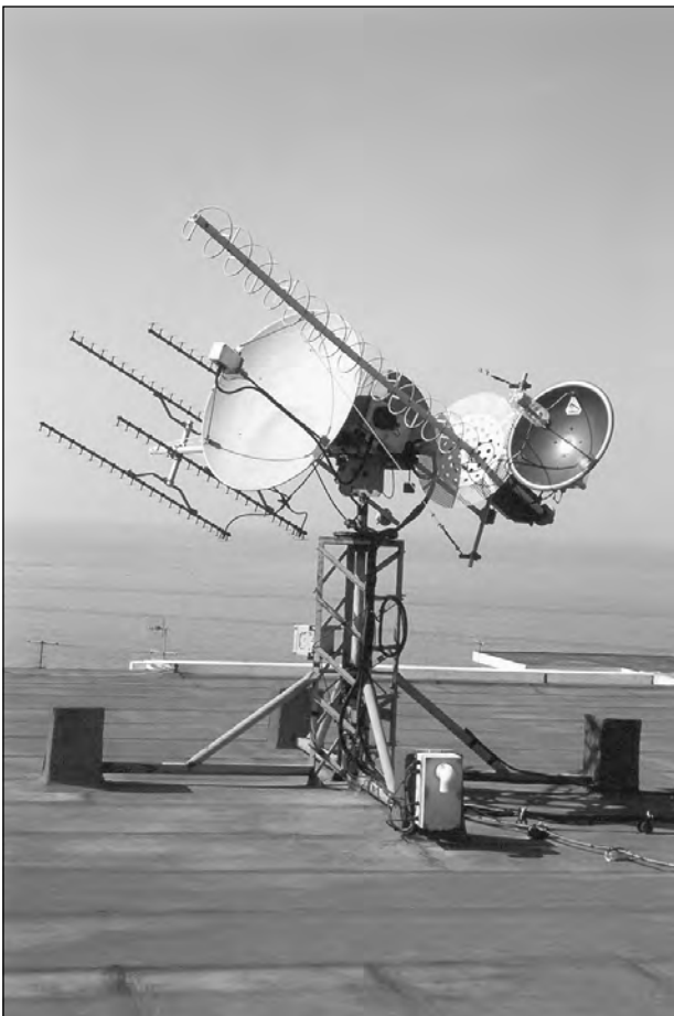
Figure 17.26 — Domenico, I8CVS, has this cluster of satellite antennas. Left to right: array of 4 \times 23 -element Yagi horizontally polarized for L band; 1.2-meter dish with 3-turn helix feed for S band; 15-turn RHCP helical antenna for U band; 60-cm dish for X band. All microwave preamplifiers and power amplifiers are homebrew and are mounted on this antenna cluster. (I8CVS photo)
