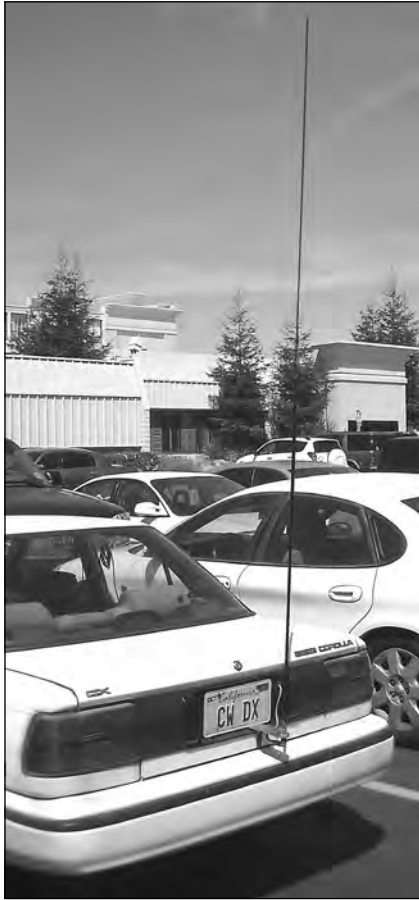
Figure 21.1 — A simple HF mobile whip can be mounted on almost any vehicle. (NØAX photo)
