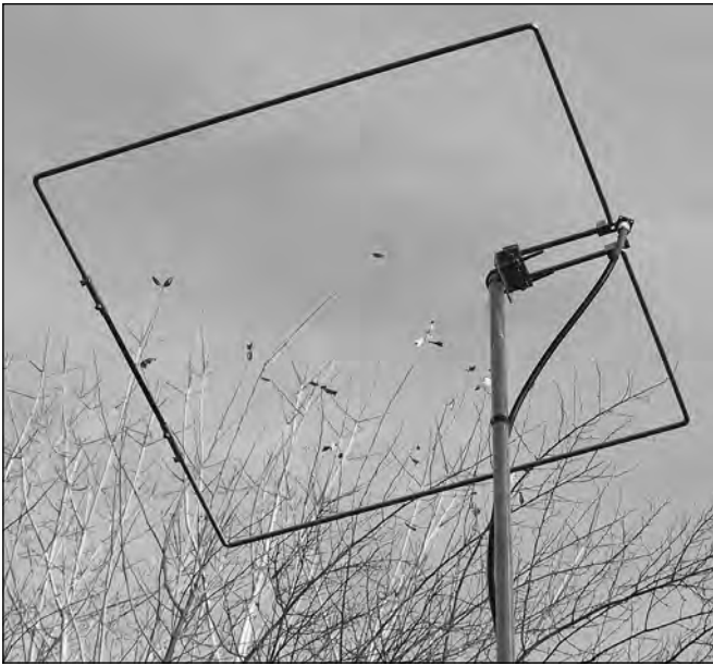
Figure 20.12 — A typical 6 meter horizontal full-wave loop antenna can be used either indoors or outdoors. The radiation pattern is omnidirectional with horizontal polarization.
