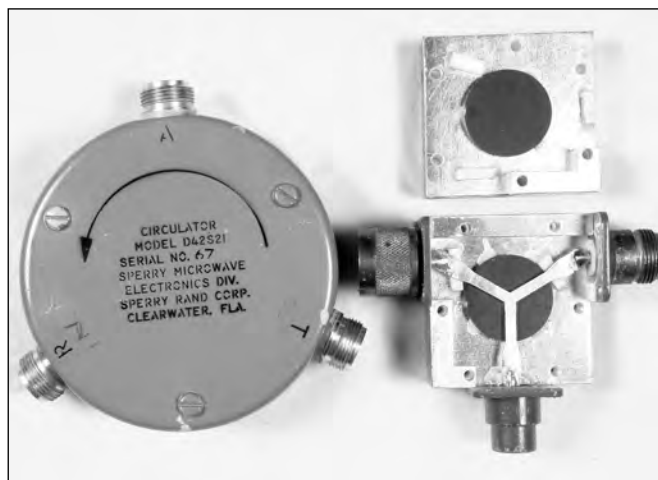
Figure 18.6 — Circulator on left has arrow showing one-way RF transmission. Isolator on right opened to show the internal construction.
