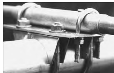
Figure 15.13 — The element to boom clamp. U bolts are used to hold the element to the plate, and 2-inch galvanized muffler clamps hold the plates to the boom.
