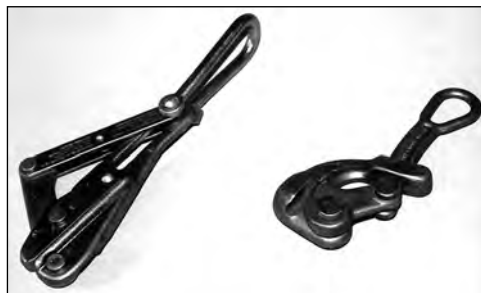
Figure 26.26 — Klein Chicago cable grip on the left and Klein Haven's grip on the right.
