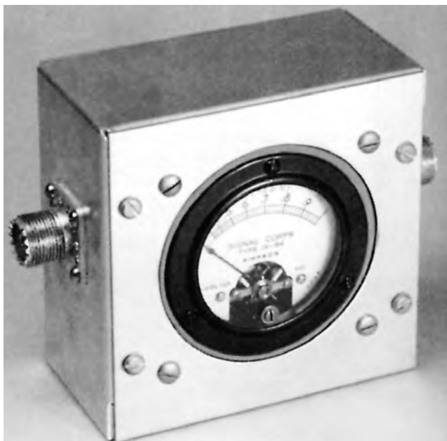
Figure 27.4 — A convenient method of mounting an RF ammeter for use in a coaxial line. This is a metal-case instrument mounted on a thin bakelite panel. The cutout in the metal clears the edge of the meter by about \frac{1}{8} inch.
