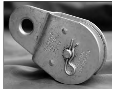
Figure 26.44 — A sturdy all-metal pulley suitable for tramping. (Don Daso, K4ZA, photo)
