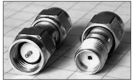
Figure 23.33 — A pair of SMA connectors, with male on the left and female on the right. SMA connectors are available in nickel, stainless steel, or gold finish.
