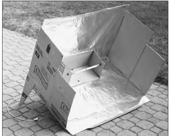
Figure 17.37 — The completed high-performance corner-reflector uplink antenna for U band. Note how the box corners hold the reflectors and dipole feed in place. The rear legs set the antenna elevation to 20° — this gives good coverage at the design latitude but will need modification for other stations.
