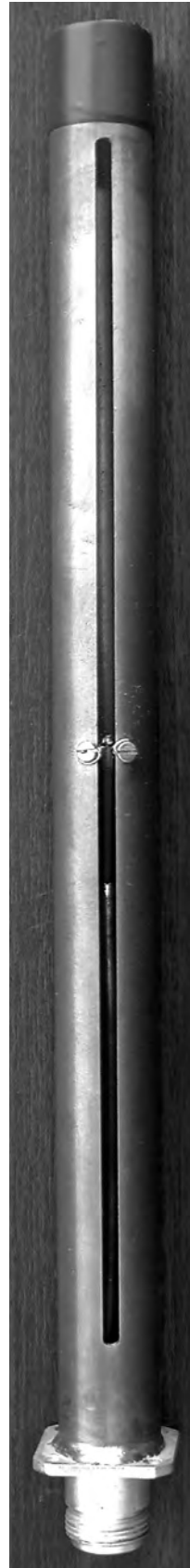
Figure 15.117 — An Alford slot antenna for 2.4 GHz made by Rob Swinbank, MØDTS.
