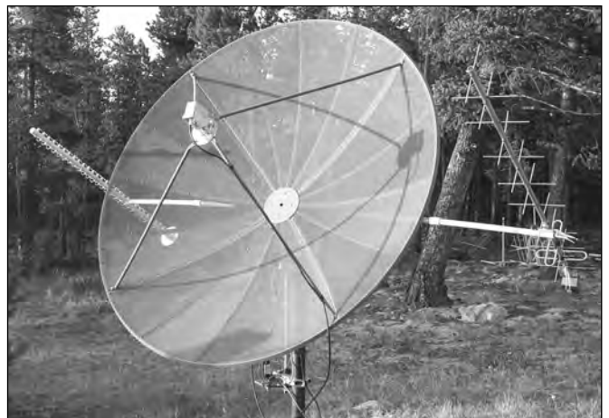
Figure 17.33 — WØLMD created this 8-foot dish with patch feed for S band for working HEO satellites. On the left is a helical antenna for L band and on the right is a 2 x 9-element offset-feed Yagi for U band. A homebrew az/el mount is provided.
