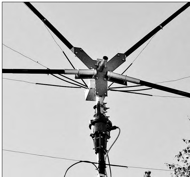
Figure 10.53 — Prototype antenna supported by trimmed cross bracket mounted atop a Yaesu G-450C rotator. A plastic box containing the 6:1 balun is mounted behind the cross bracket.
