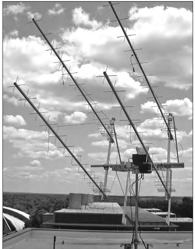
Figure 17.28 — Four-Yagi dual-polarization 432 MHz array at the Princeton University station, W2PU. The Yagis are rear-mounted; boom length is 3.5 meters, and stacking distance is 1.2 meters in each direction. (Photo courtesy Joe Taylor, K1JT)
