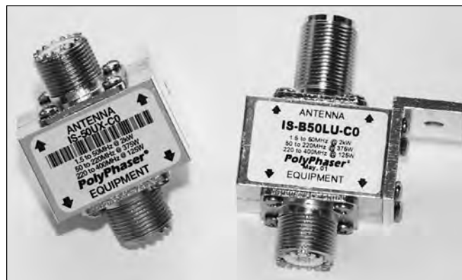
Figure 26.56 — Typical coaxial lightning arrestors from PolyPhaser. These are mounted on an cable entrance panel that is connected to a ground rod.
