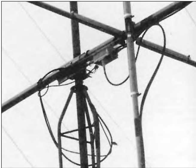
Figure 11.43 — The relay box is mounted on the boom near the center. Each of the spreader-arm fiberglass poles is attached to steel angle stock with hose clamps.
