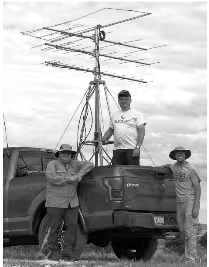
Figure 16.27 — A roof-top tripod for TV antennas is mounted in W0ZF's pickup truck on a wooden frame bolted to the bed. This also makes installing a rotator easy and even large arrays can be supported at highway speeds.
