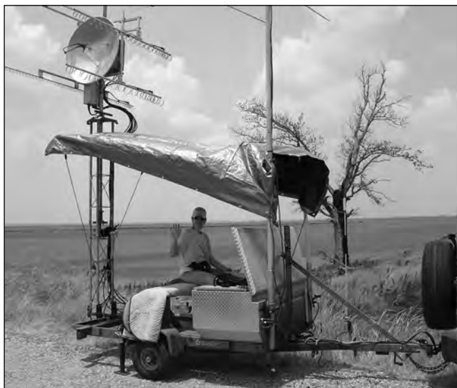
Figure 16.30 — N2CEI and K4SME mounted everything on the trailer, including the station in the heavy-duty toolbox. The trailer-mounted towers can handle substantial antennas with ease.
