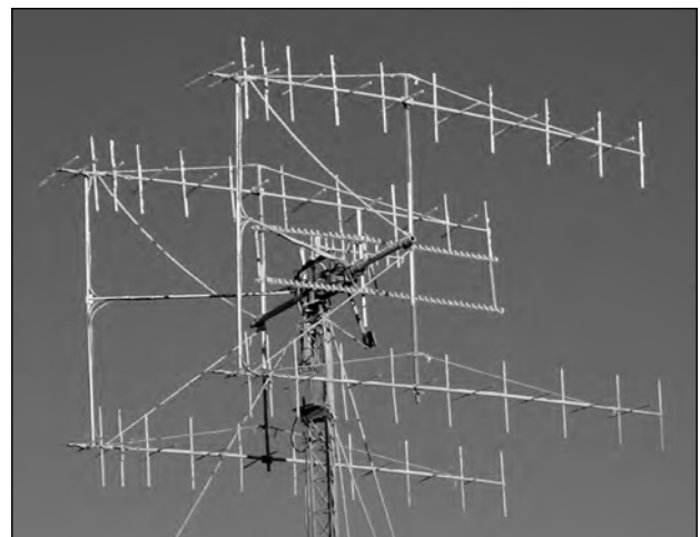
Figure 17.8 — Array of four 10-element, dual-polarization 144-MHz Yagis at KL7UW. Alaskan frost makes the horizontal and vertical elements stand out clearly. A pair of loop Yagis for 1296 MHz can be seen inside the 2 meter array.
