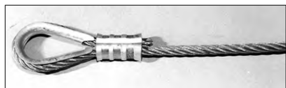
Figure 26.36 — Swaged guy wire end using Nicopress fitting.
