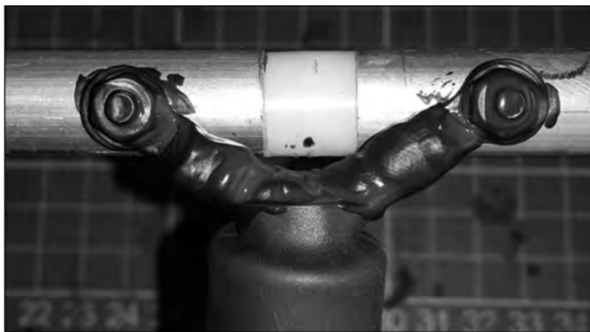
Figure 15.17 — A close-up of the feed line connection showing proper technique for creating and attaching coaxial cable to a driven element. The configuration should be as close to T-shaped as possible and in line with the element to avoid affecting performance at VHF and higher frequencies.
