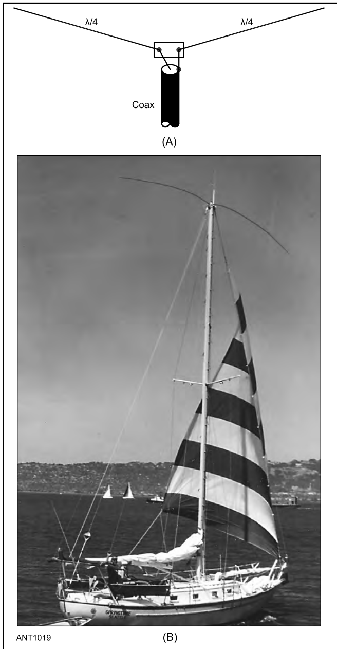
Figure 21.31 — A rigid dipole can be made from aluminum tubing, fiberglass poles or a combination of these and attached to the mast such as is visible in the photo at the top of the mast.
