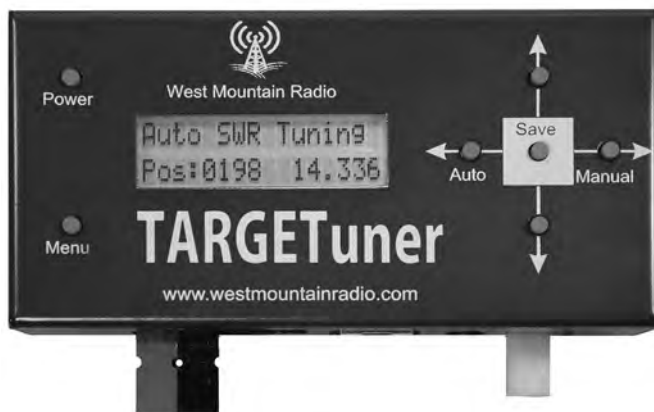
Figure 21.25 — An SWR-sensing controller adjusts the length of the screwdriver coil for minimum SWR automatically.
