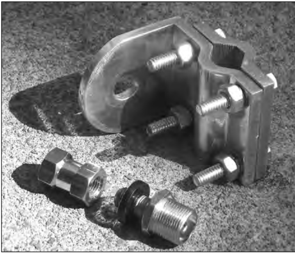
Figure 16.8 — The mirror-mount style of clamp-on bracket. This particular bracket is drilled for an SO-239 to \frac{3}{8} -24 stud mount. The bracket can be mounted on vertical or horizontal struts.
