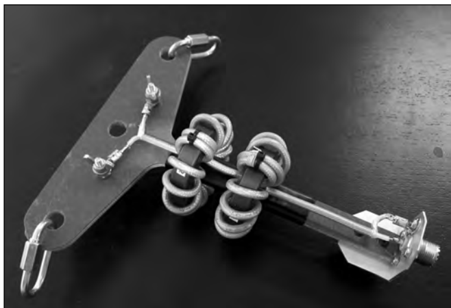
Figure 24.60 — A center insulator assembly designed by W6GJB to support one or two choke baluns in series for a wire antenna. An SO-239 is attached using a small bracket. Waterproofing can be provided by using silicone sealant.
