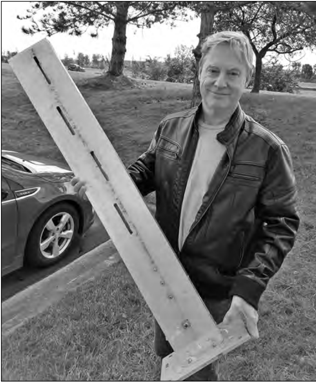
Figure 15.116 — A waveguide slot for 1296 MHz and its maker, Rene Barbeau, VE2UG.
