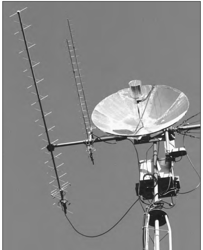
Figure 17.32 — KD1K's completed HEO antenna system mounted to the tower and ready to go. The 40 W, 23 cm amplifier is in the box below the KG6IAL 1.2 meter dish. [Dick Jansson, KD1K, photo]
