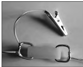
Figure 19.14 — For the multi-band dipole, antenna length and resonant frequency are changed by using alligator clips to short out insulators.
