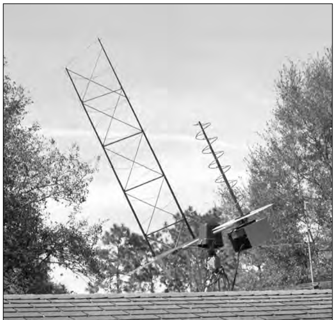
Figure 17.20 — A pair of helical antennas for service on 2 meters and 70 cm. The 2 meter helical antenna is not small!! [Dick Jansson, KD1K, photo]
