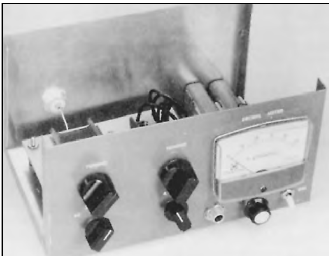
Figure 27.27 —The linear field strength meter. The control at the upper left is for C1 and the one to the right for C2. At the lower left is the band switch, and to its right the sensitivity switch. The zero-set control for M1 is located directly below the meter.
