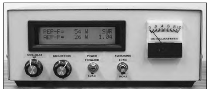
Figure 27.14 — Front panel of power meter. The LCD shows the peak envelope power (PEP), the average envelope power (AEP) and the SWR. The two knobs control the contrast and back lighting of the LCD. One toggle switch determines whether forward or load powers are displayed. A second switch sets the averaging time for the AEP calculation. The meter displays SWR and is used for tuning purposes.
