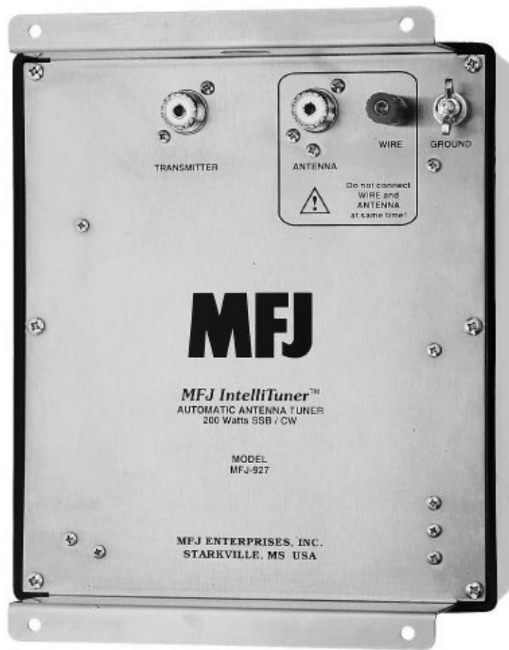
Figure 2.6 – An automatic antenna tuner will seek the best match automatically whenever you transmit. This type of tuner is extremely convenient when your antenna is located in a separate area, such as an attic. This particular model is the MFJ-927.
